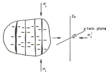
FIG. 11.—Schematic explanation of development of twin lamellae in 1046 and 1049. Detrital grain exhibits extension fractures. Movement on extension fractures is normal to fracture surfaces. This sets up a local stress ( $\sigma'_1$ ) which produces a high resolved shear stress parallel to the  $e$  twin plane and in the correct sense for twin gliding.
