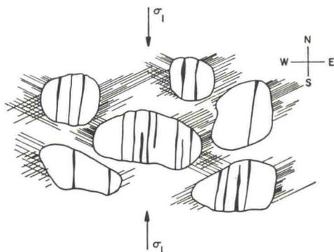
FIG. 10.—Sketch of fractured detrital grains and twin lamellae in calcite crystal. Twin lamellae are best developed on east and west sides of fractured grains and tend to die out into the interstices. Few lamellae are developed north and south of grains.
